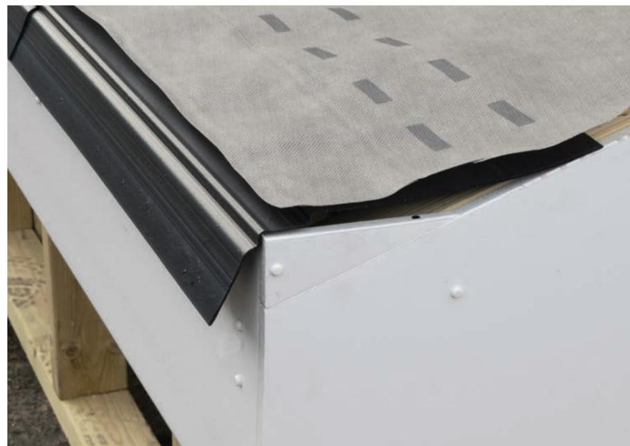
1. Lay the first layer of PERMAVENT DRY+ over the underlay support tray ensuring it finishes level with the top of the fascia and with a maximum 15mm drape between the rafters. Fix membrane to rafter with large headed tacks.
